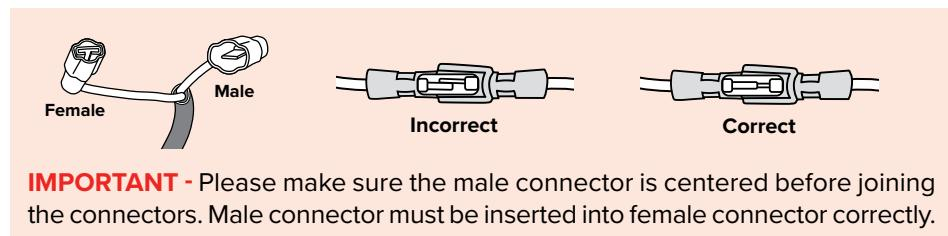
**IMPORTANT** - Please make sure the male connector is centered before joining the connectors. Male connector must be inserted into female connector correctly.
